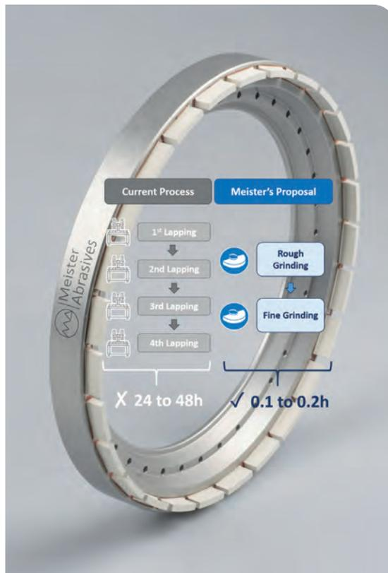
➤ Figure 3. Comparison of the standard lapping processes versus Meister coarse and ultra-fine grinding technologies.
